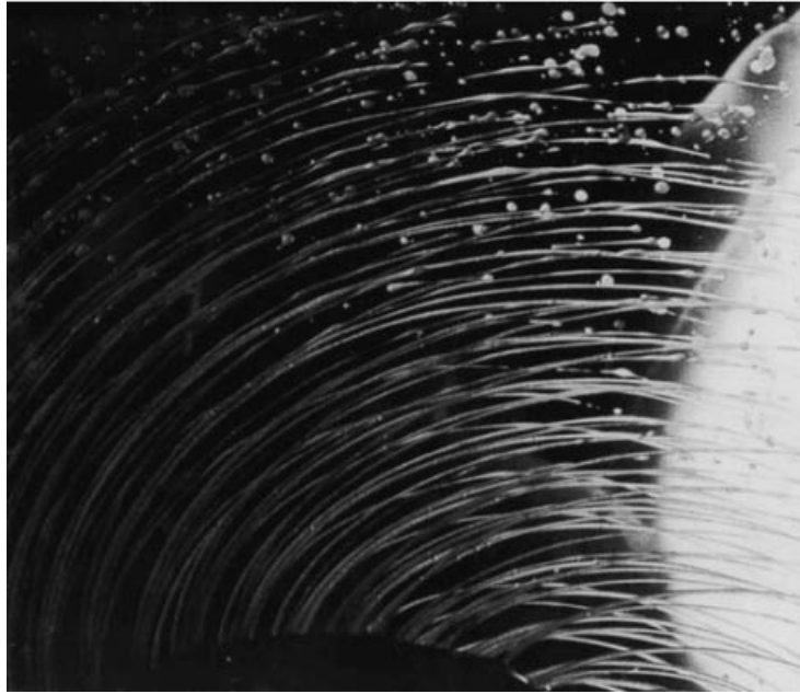
FIGURE 1. Photograph of jets emerging from a rotating container in prilling. The dark segment at the bottom of the photograph is an upper view of the rotating cylindrical container, which is rotating anticlockwise. Hundreds of jets can be seen, each emerging from small holes on the curved face of the cylinder. Some droplets, arising from jet breakup, can be observed too. The jet is seen to break up at a distance from the cylinder of the order of a hundred times the radius of a hole.
